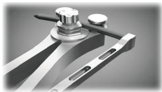
Choosing the suitable rod, using bender to pre-bending, to meet the requirement; (pay attention on the bending direction)
